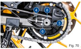
Remove the chain tensioner and push the quickrelease axle (10) to the right as much as possible (ref. Fig 71).
