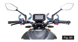
Adjust the mirror to suitable position and tighten the lock nut using a open end spanner 14 mm from the tool kit (refer page 192).
