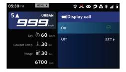
Press the 'ENT' button to 'On' or 'Off' the display call setting and to avoid the visibility of 'Display call' in the connected TET instrument cluster  If the display call setting is turned 'ON', the connected TFT instrument cluster will display the incoming call alert from the smart phone via Bluetooth. For example call from 'Arnav Kumar' will be displayed as shown below if the contact is stored in the smart phone otherwise the number will be displayed.
