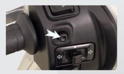
To operate the menu screens on the cluster, the HMI switch is used in the following manner:
