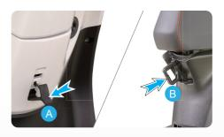
There are two bag hooks provided with your scooter to carry light luggage like carry bags weighing upto 3 kg. One hook is located below handle bar on the rear panel.
