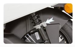
Your Scooter comes with Adjustable Shock Absorber, a first-in-the-industry feature. This allows you to adjust the required level of hardness / softness as per the usage requirement with just a push of a lever. Refer page No. 50 for details
