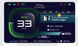
Once mobile phones connected with vehicle instrument cluster, incoming messages (1) will be shown in instrument cluster while you are riding the vehicle as shown above.
