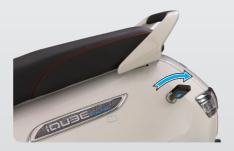
To assist you in performing certain aspects of periodic maintenance and emergency repairs, a tool kit is supplied along with the vehicle and it is located inside the utility box. To access the tool kit, insert the control key into seat lock and rotate it in clockwise direction. Lift and open the seat.
