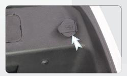
Your TVS iQube Electric S is provided with a socket for charging your smart phone even while you are traveling and it is located in the utility box below the seat assembly. Refer page No. 23 for usage details.
