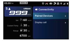
Press the 'Down' (D2) arrow of the control switches (ref. Fig. 24) and press the 'ENT' (D1) button after selecting the to 'Pair a new device' option.
