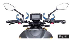
Adjust the mirror to suitable position and tighten the lock nut using a open end spanner 14 mm from the tool kit (refer page 191).
