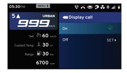
Press the 'ENT' button to 'On' or 'Off' the display call setting and to avoid the visibility of 'Display call' in the connected TET instrument cluster.
