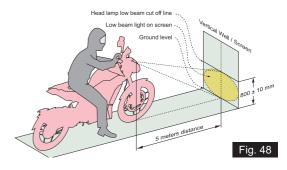
Now, turn the headlamp to low beam mode and ensure the headlamp low beam focus falls between 800 ± 10 mm from the ground level as shown (ref. Fig. 48).
