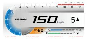
Digital bands are indicated in blue and red band based on the engine coolant temperature. Refer bellow table for details.
