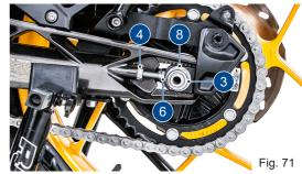
Remove the chain tensioner and push the quickrelease axle (10) to the right as much as possible (ref. Fig 72).
