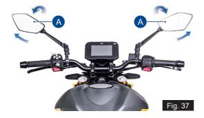
Tilt the mirror portion (A) till the clear vision is obtained (forward or backward / up or down).
