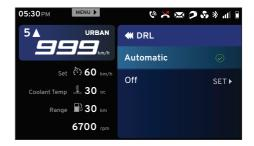
When headlamp switch is in 'Low beam' position the headlamp glows as DRL. But if the 'DRL' is turned 'OFF', the headlamp glows as 'Low beam'.  In DRL 'Automatic' condition, the DRL intensity depends on the ambient light sensor output of the connected instrument TET cluster.
