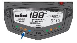
This ABS warning lamp goes 'OFF' once the bike reaches 6 km/h speed and above, and the ABS warning lamp blinks whenever the bike speed is less than 6 km/h speed indicating that the ABS is working fine.
