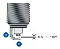
Visually inspect the spark plug gap. The gap should be 0.5 to 0.7 mm. If the gap is found to be more than the limit replace the spark plug with a new one.
