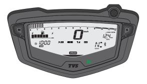
Once the cluster is connected with the smart phone, the cluster displays the signal strength of the network provider 'Tul' and the battery level 'Ull' of the smart phone. Number of unread messages 'Ull' and number of missed calls 'Ll'.
