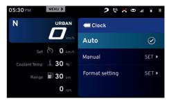
In 'Auto' mode, the clock in the connected instrument TFT cluster will get auto-synced once the mobile is connected to the cluster. Refer page 115 for detailed procedure of connecting the mobile.
