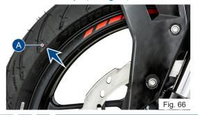
Tread depth of the tyre should be minimum 2 mm if the vehicle speed is higher than 100 km/h, and it shall be minimum 1 mm if the vehicle speed is lesser than 100 km/h
