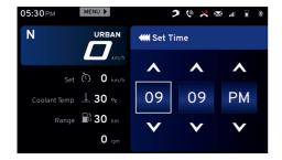
Similarly, the minute value can be adjusted by using 'Up' and 'Down' button. Pressing the 'ENT' button sets the minute and the control moves automatically to 'AM' or 'PM' selection.
