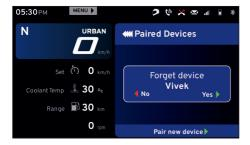
To add new device to the TFT instrument cluster, navigate to the 'Pair new device' tab and press the 'ENT' button. Refer page 115 for the detailed procedure of pairing a new device.
