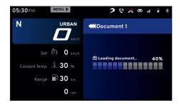
Navigate to the desired document list using 'Up' or 'Down' arrow and press the 'ENT' button to open the document.
