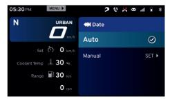
In 'Auto' mode, the date in the connected instrument TFT cluster will get auto-synced once the mobile is connected to the cluster. Refer page 115 for detailed procedure of connecting the mobile
