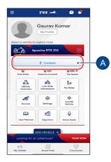
Press and hold the 'CONNECT' tab for 2 secs to erase previous vehicle details if required and connect with a new vehicle in the TVS connect app.  Press 'YES' tab to erase the previous vehicle details or 'NO' to continue as it is.
