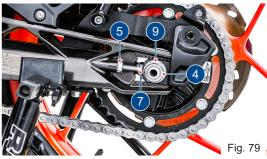
Remove the chain tensioner and push the quickrelease axle (10) to the right as much as possible (ref. Fig 80).
