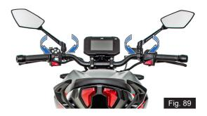
Adjust the mirror to suitable position and tighten the lock nut using a open end spanner 14 mm from the tool kit (refer page 202).
