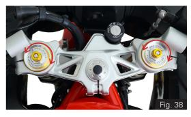
The spring preload setting is determined by the distance A or no of groove, Shorter the distance A or no of groove indicates higher preload by rotating the preload adjusting bolt clockwise, higher the distance A or no of groove indicates lower preload rotating the preload adjusting bolt anti-clockwise.
