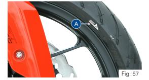
• While re-assembling the tyre, ensure that the arrow mark (1) provided on the side walls of the tyre faces the direction of wheel rotation (ref. Fig. 57)
