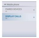
Press the 'ENT' button to 'On' or 'Off' the display call setting and to avoid the visibility of 'Display call' in the connected TFT instrument cluster.
