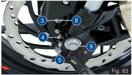
Support the front wheel and slowly pull out the quick-release axle (6) from the left side. (ref. Fig. 63).
