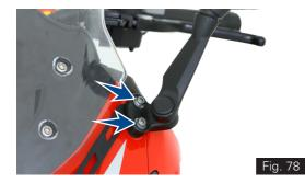
Now tighten the allen screw (2 nos) with the bracket license complete using a hexagonal key 5 mm from the tool kit (ref. Fig. 79).
