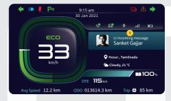
Once mobile phones connected with vehicle instrument cluster, incoming messages notification (1) will be shown in instrument cluster while you are riding the vehicle as shown above.
