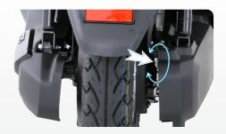
Turn the adjuster nut in clockwise direction for reducing free play or in anti-clockwise direction for increasing the free play.
