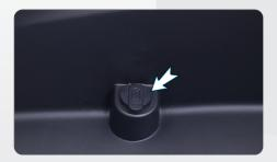
Smart phone charging socket is fitted in your TVS iQube Electric S for charging your smart phone even while you are traveling and it is located in the utility box below the seat assembly. Refer page No. 25 for usage details.
