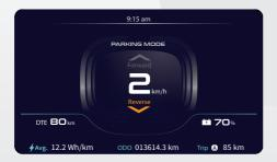
During forward movement the speed is limited to 10 km/h and during reverse speed is limited to 3 km/h
