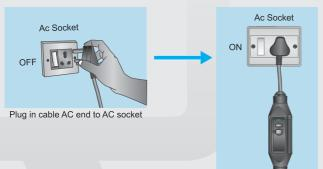
RCD Power LED will glow once the switch in AC Domestic socket is turned ON.
