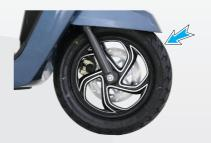
Another important unique feature in your scooter is 'Tubeless Tyres'. Tubeless tyres reduce the chances of getting punctured. Even if there is a puncture, sudden leakage of air is avoided, thereby providing better safety and convenience. It is also very easy to repair the punctured tyres.
