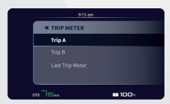
You can check the chosen trip meter readings in the display and press center button to reset the trip meter
