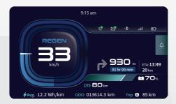
It recuperates energy lost during braking / deceleration of traction motor under specified conditions and charges the battery.
