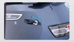
To assist you in performing certain aspects of periodic maintenance and emergency repairs, a tool kit is supplied along with the vehicle and it is located inside the utility box. To access the tool kit, insert the control key into seat lock and rotate it in clockwise direction. Lift and open the seat.
