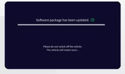
Step 8: After successful flashing, vehicle might restart depending on the controller updated. After restart wait for a minute or 2 and check for Software version in Cluster -> My vehicle -> Software -> Software
