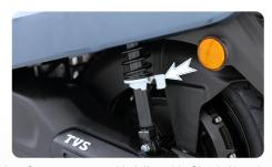
Your Scooter comes with Adjustable Shock Absorber, a first-in-the-industry feature. This allows you to adjust the required level of hardness / softness as per the usage requirement with just a push of a lever. Refer page No. 74 for details
