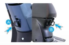
There are two bag hooks provided with your scooter to carry light luggage like carry bags weighing upto 3 kg. One hook is located below handle bar on the rear panel.
