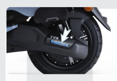
Illuminating logo will display the vehicle type name as 'ELECTRIC' during the vehicle in zero speed conditions. During charging of the vehicle, illuminating logo will blink. The LED color of the illuminating logo is Blue. Illuminating logo is mounted on the swing arm cover as shown above.
