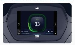
Unlike conventional scooters, this vehicle is having a digital Touch LCD / TFT instrument cluster which ensures brighter display and allows ease of interaction between vehicle and the rider.
