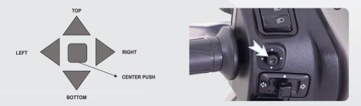
In addition to the touch screen, to operate the menu screens on the cluster, the HMI switch is used in the following manner:
