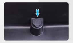
Smart phone charging socket is fitted in your TVS iQube Electric ST for charging your smart phone even while you are traveling and it is located in the utility box below the seat assembly. Refer page No. 23 for usage details.
