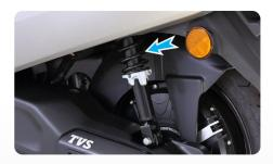
Your Scooter comes with Adjustable Shock Absorber, a first-in-the-industry feature. This allows you to adjust the required level of hardness / softness as per the usage requirement with just a push of a lever. Refer page No. 73 for details
