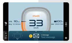
Once the smart phone is connected with the vehicle's instrument cluster, incoming messages (1) notification will be displayed on cluster as shown above.
