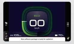
Step 5: Step 5: If the green dot is available, then proceed for flashing. Select Settings -> My vehicle -> Software -> Update -> Update. User must provide consent two times for the software flashing to initiate.
