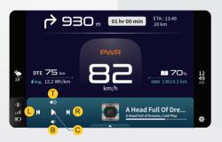
Music playing in the connected smart phone will be displayed in the instrument cluster and it can be controlled using HMI switch.
