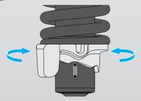
Adjust the spring pre-load by shifting the adjuster to the required notch according to the different load conditions. The more you compress the spring, the suspension becomes more stiff.
