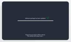
Step 8: After successful flashing, vehicle might restart depending on the controller updated. After restart wait for a minute or 2 and check for Software version in **Select Settings** -> **My vehicle** -> **Software** -> **Software Version**.
