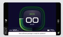
Step 5: Step 5: If the green dot is available, then proceed for flashing. Select Settings -> My vehicle -> Software -> Update -> Update. User must provide consent two times for the software flashing to initiate.
