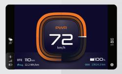
Day / Night mode can be automatically changed based on the level of ambient light. Also you can manually set the mode according to your preference.
