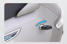
To assist you in performing certain aspects of periodic maintenance and emergency repairs, a tool kit is supplied along with the vehicle and it is located inside the utility box. To access the tool kit, insert the control key into seat lock and rotate it in clockwise direction. Lift and open the seat.
