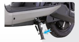
Side stand can be operated by sitting on vehicle with your left foot by pushing it away from the vehicle till it stops.
