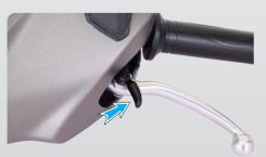
'Parking Brake' is another unique safety feature which protects your scooter from falling due to wheel rotation when it is parked with the side stand on a slope. Refer page No. 19 for details.
