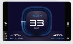
It recuperates energy lost during braking / deceleration of traction motor under specified conditions and charges the battery. Regen might not be active when the state of charge is high (higher the remaining range, lesser the regen) or when the battery temperature is high.
