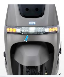
TVS iQube Electric ST comes with a Automatic Headlamp ON (AHO) LED lamp which glows automatically once the ignition is turned 'ON'.
