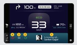
Once mobile app is connected with vehicle instrument cluster, incoming call options (1) will be shown in instrument cluster while you are riding the vehicle as shown above.
