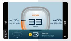
Once the smart phone is connected with the vehicle's instrument cluster, incoming messages (1) notification will be displayed on cluster as shown above.
