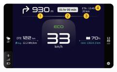
Instrument cluster displays navigation instructions of your desired destination while connected with your smart phone app, just connect and get turn by turn navigation directly on your display. It indicates the following details,
