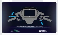
Give throttle to start the vehicle in economy mode or press mode switch again to drive in power mode.
