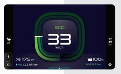
Battery level indication helps you to know how much battery charge is left in the vehicle by displaying percentage of SOC (Stage of Charge).
