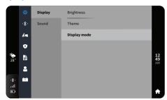
In display mode, you have the option to select between day mode, night mode, or adaptive mode. The adaptive mode enables the instrument cluster to automatically switch between day and night mode by utilizing the ambient light sensor, which detects the level of surrounding light.
