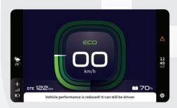
For example, if you have accelerated the scooter with brakes applied, the temperature of the motor and the MCU starts increasing. Once it reaches a critical point, the Motor Controller Unit starts "derating" the vehicle to control the increase in temperature beyond critical point, thus slowing the vehicle down a little. This may result in loss of vehicle performance to a certain extent, and you may experience some drop in performance.
