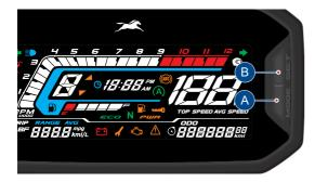
The 'Mode' (A) and 'Set' (B) buttons are provided to change between various modes and to set the some of the digital display functions of the digital speedometer. The sequence of modes and their selections are explained in detail below.
