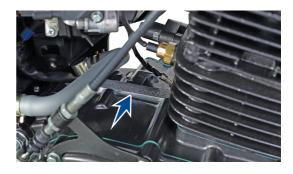
Engine serial number is stamped on the top surface of the left side crankcase assembly near the cylinder block.
