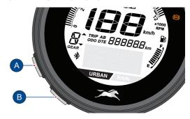
The 'Mode' (A) and 'Set' (B) buttons are provided to change between various modes and to set the some of the digital display functions of the instrument cluster. The sequence of modes and their selections are explained in detail below.
