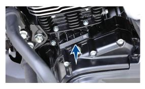
Engine serial number is engraved on the left side crankcase assembly near cylinder block as shown.
