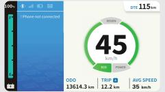
Connect with instrument cluster using mobile app to get access through various features like message notification call accept / reject options etc. on the go.
