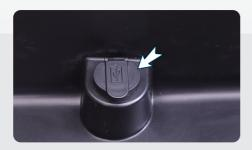
Smart phone charging socket is fitted in your TVS iQube Electric ST for charging your smart phone even while you are traveling and it is located in the utility box below the seat assembly. Refer <u>page No. 24</u> for usage details.
