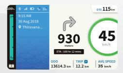
Instrument cluster displays navigation instructions of your desired destination while connected with your smart phone app, just connect and get turn by turn navigation directly on your display.
