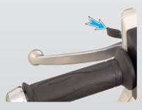
'Parking Brake' is another unique safety feature which protects your scooter from falling due to wheel rotation when it is parked with the side stand on a slope. Refer page No. 18 for details.
