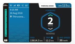
Press park assist switch once again, for shifting to reverse mode as shown, apply throttle to move.
