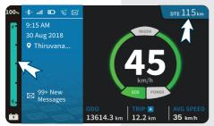
Battery level indication helps customer to know how much battery charge is left in the vehicle by displaying percentage of SOC (Stage of Charge).
