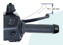
Turn the adjuster nut at the bottom side
