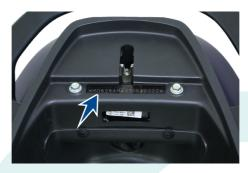
The frame serial number is stamped on the frame, at the rear end below the seat assembly. Open the seat assembly to read the frame number.
