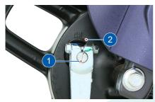
Incase the wear limit index mark (1) is going beyond wear limit indicator (2), index the lever to next slot with the help of the Dealer to extend the shoe life.
