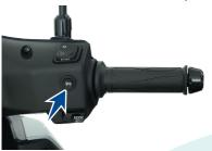
The vehicle will enter into park assist forward mode as indicated on the cluster, apply throttle to move forward.
