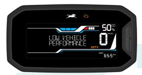
To ensue the safety of you and your TVS Orbiter, in high temperature condition, overloaded condition or continuous peak performance usage whenever the temperature of vehicle components reaches a critical point, as a safety measure performance of some systems are deliberately reduced to optimize the temperature. This is indicated by the MIL on your dashboard glowing after sometime accompanied by a message.
