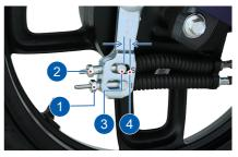
If any clearance is found, turn the adjuster nut (2) at the top side in the slot marked as 'S' in clockwise direction until there is no clearance between the bullet top (3) and the slot top (4).
