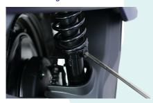
Adjust the spring pre-load by shifting the adjuster to the required notch according to the different load conditions. The more you compress the spring, the suspension becomes more stiff.
