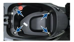
4. Take out the utility box along with the seat while carefully disconnecting the wiring socket of utility box lamp and diagnostic coupler (please note that the seat comes along with utility box since it is mounted on the utility box).
