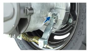
Reassemble the oil level bolt with new fiber washer.
