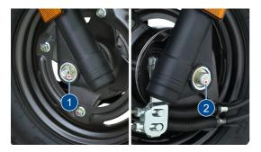
6. Reverse the procedure for reassembling, while ensuring the proper seating of brake panel slot in the fork leg L lug (LH side) and hub drive lugs in the slots of wheel hub (RH side).
