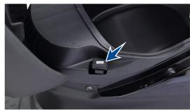
Turn 'ON' the ignition lock and check for proper functioning of electrical systems. Incase the fuse fails again, consult the nearest TVS Motor Company Authorised Main Dealer / Authorised Dealer
