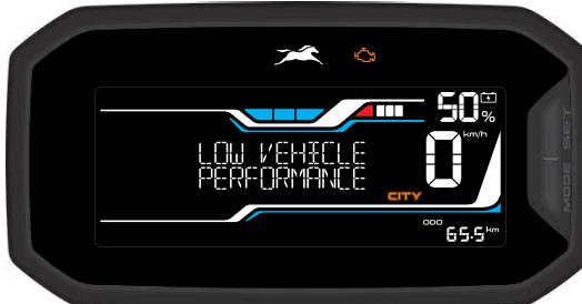
To ensure the safety of you and your TVS Orbiter, in high temperature condition, overloaded condition or continuous peak performance usage whenever the temperature of vehicle components reaches a critical point, as a safety measure performance of some systems are deliberately reduced to optimize the temperature. This is indicated by the MIL on your dashboard glowing after sometime accompanied by a message.
