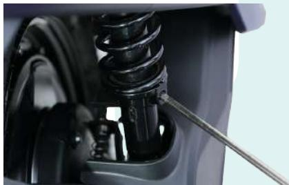
Adjust the spring pre-load by shifting the adjuster to the required notch according to the different load conditions. The more you compress the spring, the suspension becomes more stiff.
