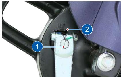
In case the wear limit index mark (1) is going beyond wear limit indicator (2), index the lever to next slot with the help of the Dealer to extend the shoe life.
