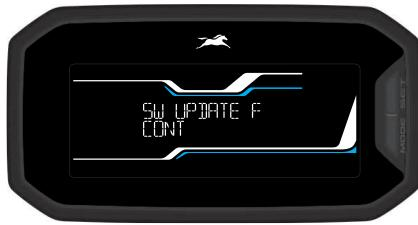
1. If OTA update has failed, Cluster will display Software installation failed message and screen will transform to idle screen after 5 seconds.
