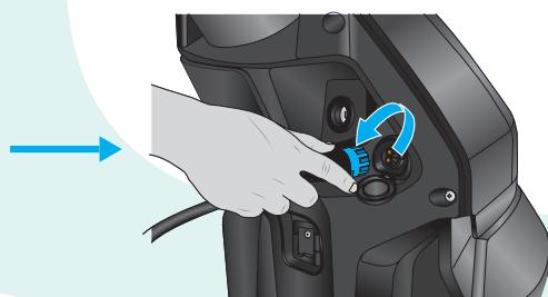
Rotate counter clock wise to plug out cable other end from vehicle charging socket & close vehicle charging socket cap
