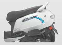
To assist you in performing certain aspects of periodic maintenance and emergency repairs, a tool kit is supplied along with the vehicle and it is located inside the utility box. To access the tool kit, insert the control key into seat lock and rotate it in clockwise direction. Lift and open the seat.
