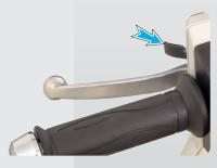
'Parking Brake' is another unique safety feature which protects your scooter from falling due to wheel rotation when it is parked with the side stand on a slope. Refer page No. 19 for details.
