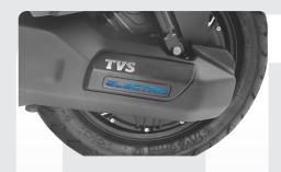
Illuminating logo will display the vehicle type name as 'ELECTRIC' during the vehicle in zero speed conditions. During charging of the vehicle, illuminating logo will blink. The LED color of the illuminating logo is Blue. Illuminating logo is mounted on the swing arm cover as shown above.
