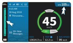
Battery level indication helps customer to know how much battery charge is left in the vehicle by displaying percentage of SOC (Stage of Charge).
