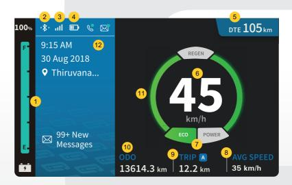
Battery level indicator (SOC) -Indicates battery charge in percentage as well as bars:
