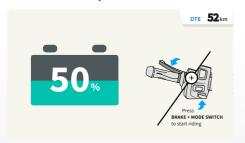
Give throttle to start the vehicle in economy mode or press mode switch again to drive in power mode.
