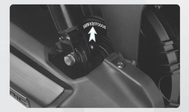
The traction motor serial number is stamped on the hub of the rear wheel assembly. Rotate the rear wheel assembly to read the motor number.
