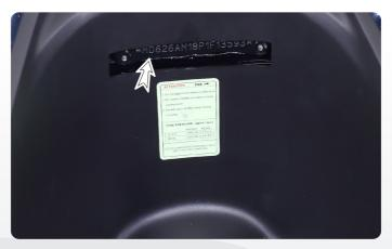
The frame serial number is stamped on the frame, at the rear end below the seat assembly. Open the seat assembly and remove the VIN cover to read the frame number.
