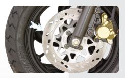
Taking technological innovation to next level, your scooter comes with 'Synchronised Brake Technology (SBT)'. This feature enhances the safety by avoiding skidding during sudden braking.
