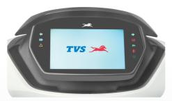
Unlike conventional scooters this vehicle is having a digital instrument cluster which ensures brighter display and allows ease of interaction between vehicle and customer.
