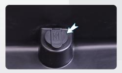
Smart phone charging socket is fitted in your TVS iQube Electric ST for charging your smart phone even while you are traveling and it is located in the utility box below the seat assembly. Refer <u>page No. 25</u> for usage details.
