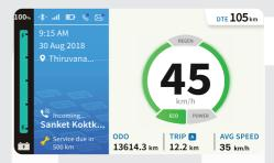
Once Mobile phone is connected with vehicle instrument cluster, incoming call options and messages will be shown in instrument cluster while customer is riding the vehicle as shown above.
