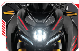
CLASS D PROJECTOR HEADLAMP WITH LED DRLs
