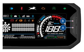
The 'Mode' (A) and 'Set' (B) buttons are provided to change between various modes and to set the some of the digital display functions of the digital speedometer. The sequence of modes and their selections are explained in detail below.
