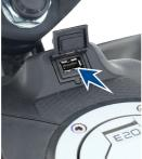
3. Do make sure the flap is not damaged while opening / inserting the USB cable.
