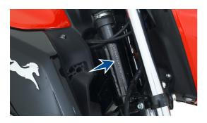
The frame serial number is stamped on the right side of the steering head tube.
