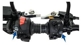
'Info switch' is located at the left side of the handle bar. 'Info switch' is used erase the stored value in cluster / to accept or reject the incoming call , also ongoing call can be ended. Low fuel auto navigation can be accepted or rejected etc.
