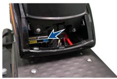
Turn 'ON' the ignition lock and check for proper functioning of the electrical systems. Incase the fuse fails again, consult the nearest TVS Motor Company Authorised Main Dealer / Authorised Dealer.
