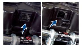
Do make sure the flap is not damaged while opening / inserting the USB cable.
