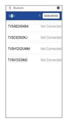
Press and hold "CONNECT" for 2 sec to erase previous vehicle details and connect with a new vehicle in the TVS connect app.
