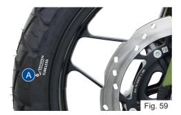
While re-assembling the tyre, ensure that the arrow mark (1) provided on the side walls of the tyre faces the direction of wheel rotation (ref. Fig. 59).
