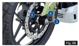
Support the front wheel and slowly pull out the quick-release axle (4) from the left side. (ref. Fig. 67).
