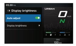
When Display brightness mode is selected, the user can set to various levels based on your preference by using 'Up' (e2) or 'Down' (e3) arrow.
