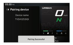
Once device is paired, the Bluetooth ' ≯ ' icon, Wi-fi ' ? ' icon once enabled, phone's battery ' î ' icon and signal strength ' ₁ 1 ' icons will be displayed on the connected instrument cluster.
