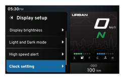
The 'Clock setting' features allows you to adjust the clock timing of your connected instrument TFT cluster. The 'Clock setting' feature has three settings and they are:
