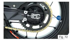
Carefully roll the rear wheel out from the swing arm while pulling the brake-caliper assembly back far enough to allow the rear wheel to come out.
