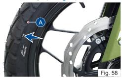
Tread depth of the tyre should be minimum 2 mm if the vehicle speed is higher than 100 km/h, and it shall be minimum 1 mm if the vehicle speed is lesser than 100 km/h
