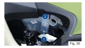
Contact TVS Motor Company Authorised Main Dealer for topping-up if the level in the tank is lower than the minimum level
