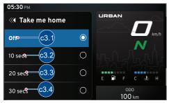
Using 'Up' (e2) or 'Down' (e3) arrow either you can alter the duration of headlamp 'ON' timing or you can switch 'OFF' the take me home function
