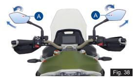
Tilt the mirror portion (A) till the clear vision is obtained (up or down).
