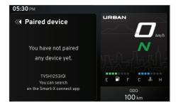
To add new device to the TFT instrument cluster, navigate to the 'Paired device' tab and press the 'ENT' button. Refer page 75 for the detailed procedure of pairing a new device. A new device can also be paired directly from Home screen by selecting device name in App.
