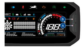
The 'Mode' (A) and 'Set' (B) buttons are provided to change between various modes and to set the some of the digital display functions of the digital speedometer. The sequence of modes and their selections are explained in detail below.
