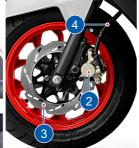
3. If the brake fluid level is below the mark or while applying brake if you feel the brake is more spongy or ineffective due to air entry, contact TVS Motor Company Authorised Main Dealer or Authorised Dealer for topping-up the brake fluid, air bleeding and other brake related inspections.
