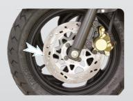
Taking technological innovation to next level, your scooter comes with 'Synchronised Brake Technology (SBT)'. This feature enhances the safety by avoiding skidding during sudden braking.
