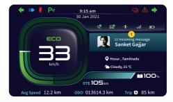
Once mobile phones connected with vehicle instrument cluster, incoming messages (1) will be shown in instrument cluster while you are riding the vehicle as shown above
