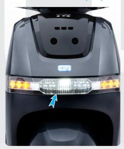
TVS iQube Electric S comes with a Automatic Headlamp ON (AHO) LED lamp which glows automatically once the ignition is turned 'ON'.
