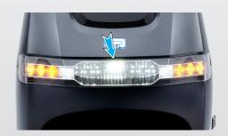
Your Scooter comes in with premium LED lamps. Efficient and bright, this gives TVS iQube Electric S a totally upgraded Look and Style with better visibility for night rides. LED lamps consume less power with increased luminous intensity.
