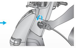
Rotate counter clock wise to plug out cable other end from vehicle charging socket & close vehicle charging socket cap
