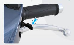
'Parking Brake' is another unique safety feature which protects your scooter from falling due to wheel rotation when it is parked with the side stand on a slope. Refer page No. 17 for details.
