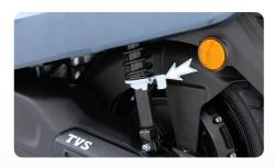
Your Scooter comes with Adjustable Shock Absorber, a first-in-the-industry feature. This allows you to adjust the required level of hardness / softness as per the usage requirement with just a push of a lever. Refer page No. 50 for details
