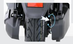
4. Turn the adjuster nut in clockwise direction for reducing free play or in anti-clockwise direction for increasing the free play.
