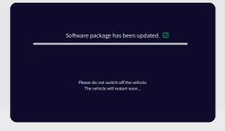
Step 8: After successful flashing, vehicle might restart depending on the controller updated. After restart wait for a minute or 2 and check for Software version in Cluster -> My vehicle -> Software -> Software
