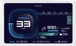
It recuperates energy lost during braking / deceleration of traction motor under specified conditions and charges the battery.
