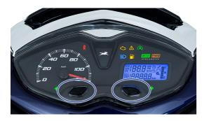
The multifunction display of the speedometer has various functions like 'ODO', 'TRIP A', 'TRIP B', 'TRIP F#', 'DTE##', 'AFE', 'IFE' and 'CLOCK'.
