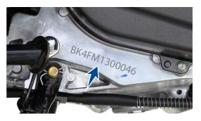
The engine serial number is stamped on the left side of the engine, at the bottom, near center stand mounting. See bottom to read serial number.
