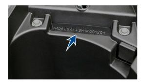
The frame serial number is stamped on the frame, at the rear end below the seat assembly. Open the seat assembly to read the frame number.
