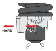
Adjust the spring pre-load by shifting the adjuster to the required notch according to the different load conditions. The more you compress the spring, the suspension becomes more stiff.
