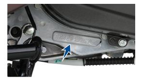
The engine serial number is stamped on the left side of the engine, at the bottom, near center stand mounting. See bottom to read serial number.
