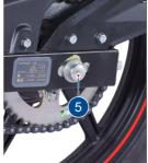
For locating and reassembling the rear wheel easily, engage the gear. This will arrest the free movement of the drum sprocket. Reverse the procedure for reassembly.
