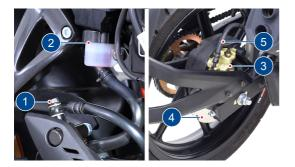
3. If the brake fluid level is below minimum or while applying brake if you feel the brake is more spongy or ineffective due to air entry, contact TVS Motor Company Authorised Main Dealer / Authorised Dealer for topping-up the brake fluid, air bleeding and other brake related inspections.
