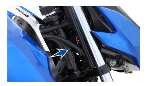
Frame serial number is engraved on the right side of the steering head tube as shown.
