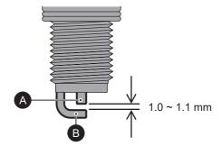
After cleaning and adjusting the gap, reinstall the spark plug and tighten by hand to avoid cross threading. Finally tighten using spark plug spanner.
