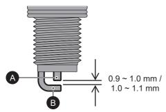
A spark plug with heavy carbon deposits will not produce strong sparks. Hence, only if necessary, clean the carbon deposits from the spark plug with a small wire brush or spark plug cleaning tool.
