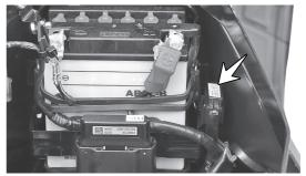
Turn 'ON' the ignition lock and check for proper functioning of electrical systems. Incase the fuse fails again, consult the nearest TVS Motor Company Authorised Main Dealer / Authorised Dealer.
