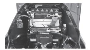
Reinstall the filler caps and clean the battery thoroughly, apply petroleum jelly to the battery terminals to protect it from corrosion.
