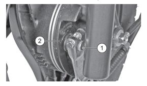
Incase the wear limit index mark (1) is going beyond wear limit indicator (2), index the lever to next slot with the help of the Dealer to extend the shoe life.
