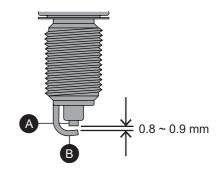
Visually inspect the spark plug gap. The gap should be 0.8 to 0.9 mm. If the gap is found to be more than the limit replace the spark plug with a new one.
