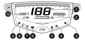
1. Speedometer Indicates the vehicle speed in kilometer per hour.
