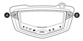
The Mode (A) and Set (B) buttons are provided to change between various modes and to set the some of the digital display functions of the instrument cluster. The sequence of modes and their selections are explained in detail below.
