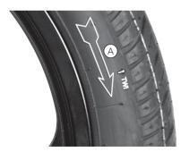
While reassembling the tyre, after removing from the wheel rim, ensure that the arrow mark (A) on the tyre facing the direction of wheel rotation.
