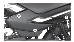
Open the cover frame L in the following manner to access the battery assembly.
