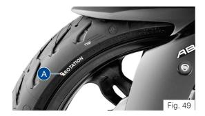
While re-assembling the tyre, ensure that the arrow mark (1) provided on the side walls of the tyre faces the direction of wheel rotation (ref. Fig. 49).
