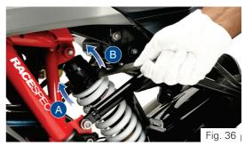
To adjust the shock absorber's pre-load:
