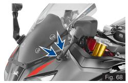
Now tighten the allen screw (2 nos) with the bracket licence complete using a hexagonal key 5 mm from the tool kit (ref. Fig. 69).
