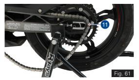
Carefully roll the rear wheel out from the swing arm while pulling the brake-caliper assembly back far enough to allow the rear wheel to come out.
