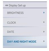
In the connected TFT instrument cluster, with the help of photo sensor, the Day & Night mode themes will be changed automatically.
