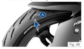
Tread depth of the tyre should be minimum 2 mm if the vehicle speed is higher than 100 kmph, and it shall be minimum 1 mm if the vehicle speed is lesser than 100 kmph.
