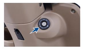
To lock the steering, turn the handle bar all the way to the 'left' or 'right'. Push the key 'IN', turn it to the 'LOCK' position and take out. All the electrical circuits are turned 'OFF' in this position. Insert the key into the lock and turn it to 'OFF' or 'ON' position to unlock the steering.
