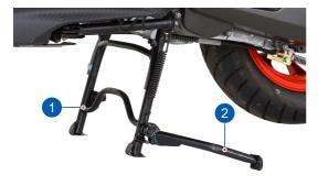
To place the vehicle on centre stand, hold the handle bar left grip with left hand, place your foot firmly on the centre stand extension (2) while ensuring that both the stand shoes are touching the ground, press the stand extension.
