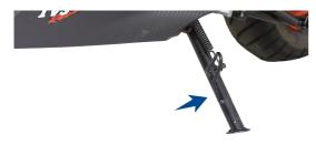
Side stand can be operated by sitting on vehicle with your left foot by pushing it away from the vehicle till it stops.
