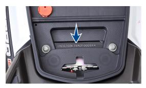
The frame serial number is stamped on the frame, at the rear end below the seat assembly. Open the seat assembly to read the frame number.
