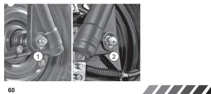
6. Reverse the procedure for reassembling, while ensuring the proper seating of brake panel slot in the fork leg L lug (LH side) and hub drive lugs in the slots of wheel hub (RH side)
