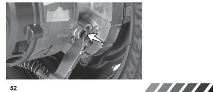
6 Reassemble the oil level bolt with new fiber washer
