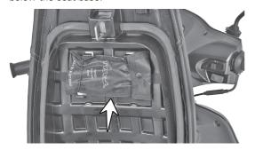
Lift the seat by unlocking the seat lock as explained in page no. 16, to access the tool kit. The tool kit consists one number each of the following. Ensure the contents of tool kit.
