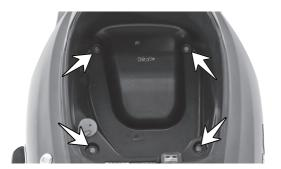
3. Take out the utility box along with the seat while carefully disconnecting the wiring socket of utility box lamp and diagnostic coupler (please note that the seat comes along with utility box since it is mounted on the utility box).
