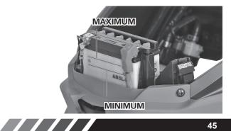
While connecting the terminals, observe the correct polarity. Connect the red wire to the '+' terminal and black wire to the '-' terminal of the battery.
