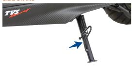
Side stand can be operated by sitting on vehicle with your left foot by pushing it away from the vehicle till it stops.
