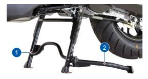
To place the vehicle on centre stand, hold the handle bar left grip with left hand, place your foot firmly on the centre stand extension (2) while ensuring that both the stand shoes are touching the ground, press the stand extension.
