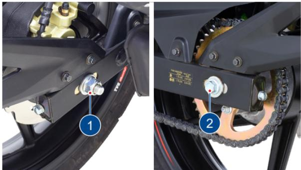
3. Take out the caliper assembly by dislocating it from the disc and the swing arm lug.
