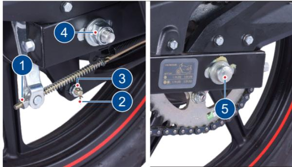
6. For locating and reassembling the rear wheel easily, engage the gear. This will arrest the free movement of the drum sprocket. Reverse the procedure for reassembly.
