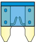
4. The fuse box contains two 15A fuses and one 10A fuse. One 15A fuse is used for ABS system while the other one is used for DC loads. 10A fuse is used for EMS system. Use the fuse puller (A) placed near the fuse box to pull out the blown fuse.
