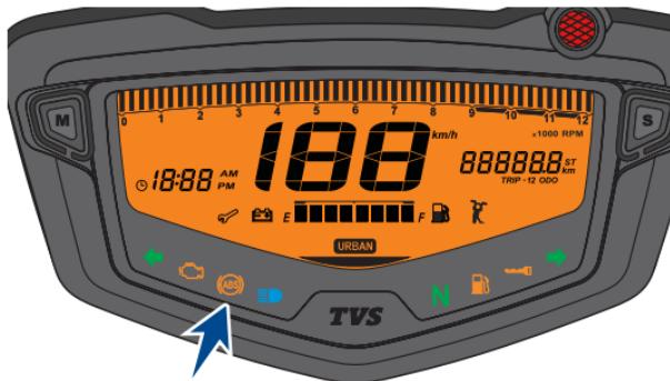
This ABS warning lamp goes 'OFF' once the bike reaches 6 km/h speed and above and the ABS warning lamp blinks whenever the bike speed is less than 6 km/h speed indicating that the ABS is working fine.
