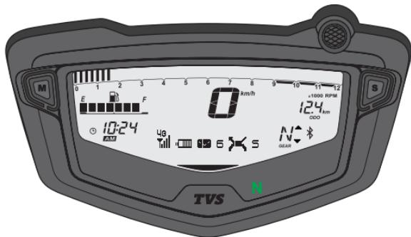
Once the cluster is connected with the smart phone, the cluster displays the signal strength of the network provider '4G' and the battery level '█' of the smart phone. Number of unread messages '✉ 6' and number of missed calls 'missed'.
