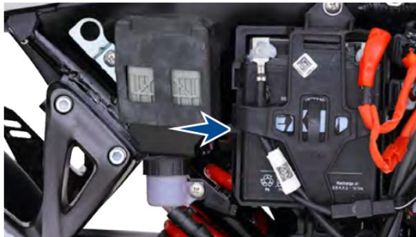
4. While connecting the terminals, observe the correct polarity. Connect the red wire to the '+' terminal and black wire to the '-' terminal of the battery.
