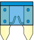
4. The fuse box contains one 15A fuse, one 10A fuse and one 20A fuse. The 20A fuse is used for dual channel ABS system. Incase of single channel ABS system, 15A fuse is provided instead of 20A fuse. 15A fuse used for DC loads and 10A fuse used for EMS. Use the 'fuse puller' (A) placed near the fuse box to pull out the blown fuse.
