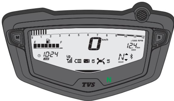
Once the cluster is connected with the smart phone, the cluster displays the signal strength of the network provider '4G' and the battery level '■■■■' of the smart phone. Number of unread messages '✉ 4' and number of missed calls 'missed calls'.
