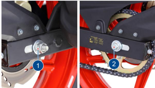
2. Take out the caliper assembly by dislocating it from the disc and the swing arm lug.
