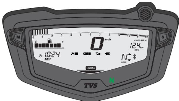
Once the cluster is connected with the smart phone, the cluster displays the signal strength of the network provider '  $\text{T}_{\text{ll}}$  ' and the battery level '  $\text{B}_{\text{ll}}$  ' of the smart phone. Number of unread messages '  $\text{M}_{\text{ll}}$  ' and number of missed calls '  $\text{X}_{\text{ll}}$  '.
