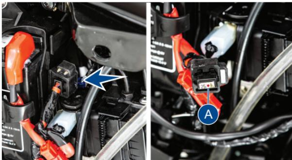
3. Replace the blown fuse with a new one with the same rating (extra fuse (A) is provided in the fuse holder itself).
