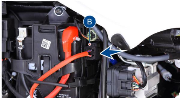
3. Replace the blown fuse with a new one with the same rating (extra fuse is provided in the fuse holder itself).
