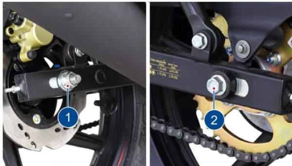
2. Take out the caliper assembly by dislocating it from the disc and the swing arm lug. Carefully hang the caliper assembly in the swing arm itself.
