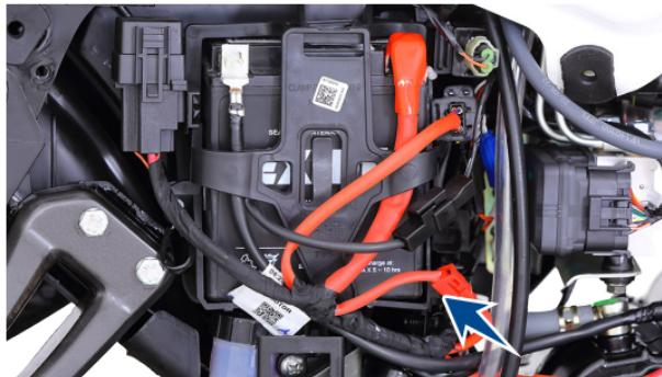
3. While connecting the terminals, observe the correct polarity. Connect the red wire to the '+' terminal and black wire to the '-' terminal of the battery.
