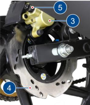
3. If the brake fluid level is below minimum or while applying brake if you feel the brake is more spongy or ineffective due to air entry, contact TVS Motor Company Authorised Main Dealer / Authorised Dealer for topping-up the brake fluid, air bleeding and other brake related inspections.
