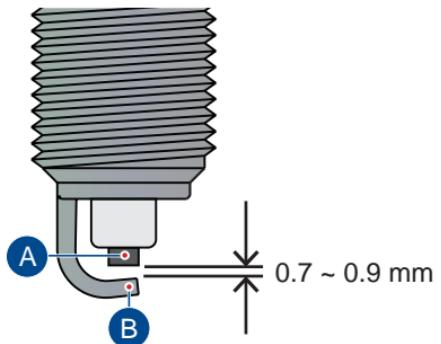
Inspect the spark plug gap visually (0.7 ~ 0.9 mm). If the gap is found to be more, replace the spark plug with a new one.
