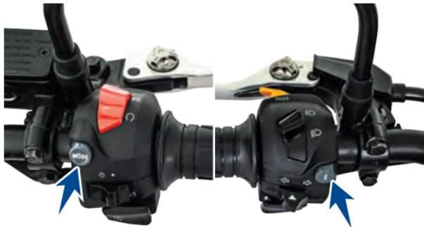
'Info switch' is located at the left side of the handle bar. 'Info switch' is used to erase the stored value in cluster / to accept or reject the incoming call / voice assist invoking, also ongoing call can be ended. Low fuel auto navigation can be accepted or rejected etc.
