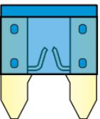
4. The fuse box contains one 15A fuse, one 10A fuse and one 20A fuse. The 20A fuse is used for dual channel ABS system. Incase of single channel ABS system, 15A fuse is provided instead of 20A fuse. 15A fuse used for DC loads and 10A fuse used for EMS. Use the 'fuse puller' (A) placed near the fuse box to pull out the blown fuse.
