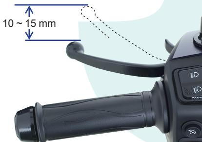
3. If the measured distance is more than the limit, adjust the nut provided at the rear wheel end to obtain the correct play.
