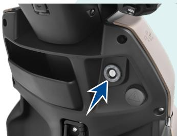
To lock the steering, turn the handle bar all the way to the 'left' or 'right'. Push the key 'IN', turn it to the 'LOCK' position and take out. All the electrical circuits are turned 'OFF' in this position. **Insert the key into the lock and turn it to 'OFF' or 'ON' position to unlock the steering.**
