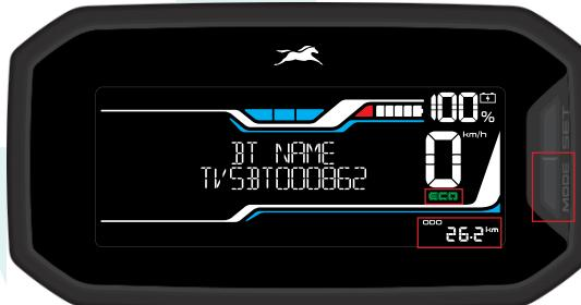
4. Open the 'TVS CONNECT' app login with credentials and press the 'CONNECT' tab, while ensuring that the smart phone is near to the vehicle and Bluetooth is turned On.
