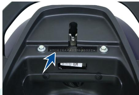
The frame serial number is stamped on the frame, at the rear end below the seat assembly. Open the seat assembly to read the frame number.
