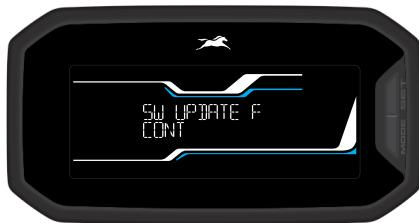
1. If OTA update has failed, Cluster will display Software installation failed message and screen will transform to idle screen after 5 seconds.
