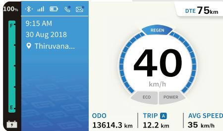
It recuperates energy lost during braking / deceleration of traction motor under specified conditions and charges the battery. Regen is a natural phenomena, it does not require to select any mode and screen changes to Regen as shown above automatically and reverts back to drive mode screen when regen deactivates.
