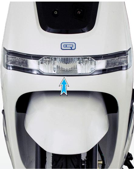
TVS iQUBE ELECTRIC SMARTXONNECT 9 comes with a Automatic Headlamp ON (AHO) LED lamp which glows automatically once the ignition is turned 'ON'.
