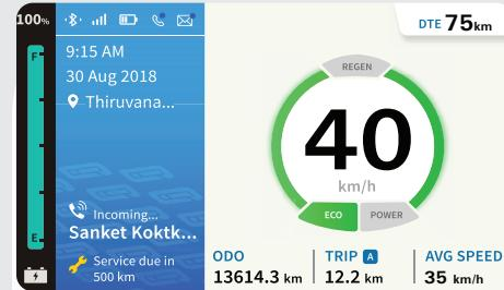
Once Mobile phone is connected with vehicle instrument cluster, incoming call options and messages will be shown in instrument cluster while customer is riding the vehicle as shown above.
