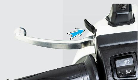
'Parking Brake' is another unique safety feature which protects your scooter from falling due to wheel rotation when it is parked with the side stand on a slope. Refer [page No. 19](#) for details.
