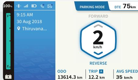
It reduces the effort of parking for customer by allowing controlled movement of the vehicle in forward or reverse direction with minimal speed.
