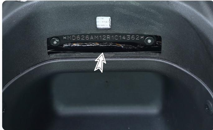
The frame serial number is stamped on the frame, at the rear end below the seat assembly. Open the seat assembly and remove the VIN cover to read the frame number.
