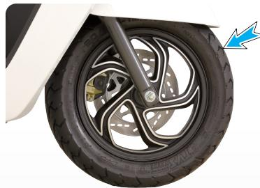
Another important unique feature in your scooter is 'Tubeless Tyres'. Tubeless tyres reduce the chances of getting punctured. Even if there is a puncture, sudden leakage of air is avoided, thereby providing better safety and convenience. It is also very easy to repair the punctured tyres.
