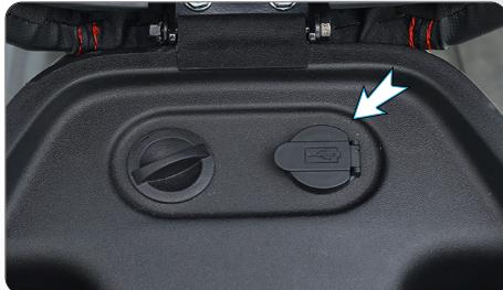
Your TVS iQUBE ELECTRIC SMARTXONNECT 9 is provided with a socket for charging your smart phone even while you are traveling and it is located in the utility box below the seat assembly. Refer [page No. 25](#) for usage details.
