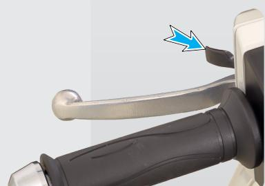
'Parking Brake' is another unique safety feature which protects your scooter from falling due to wheel rotation when it is parked with the side stand on a slope. Refer [page No. 19](#) for details.
