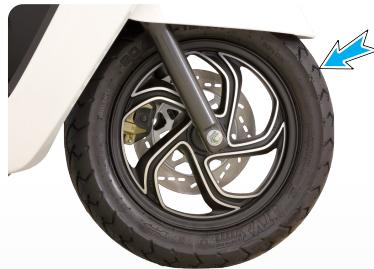
Another important unique feature in your scooter is 'Tubeless Tyres'. Tubeless tyres reduce the chances of getting punctured. Even if there is a puncture, sudden leakage of air is avoided, thereby providing better safety and convenience. It is also very easy to repair the punctured tyres.
