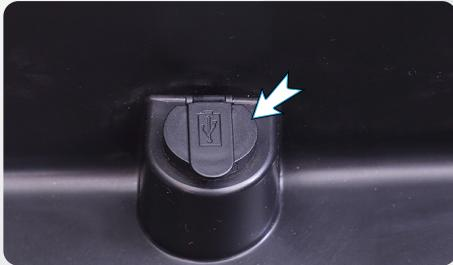
Smart phone charging socket is fitted in your TVS iQube Electric ST for charging your smart phone even while you are traveling and it is located in the utility box below the seat assembly. Refer [page No. 25](#) for usage details.
