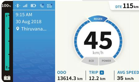
It recuperates energy lost during braking / deceleration of traction motor under specified conditions and charges the battery. Regen is a natural phenomena, it does not require to select any mode and screen changes to Regen as shown above automatically and reverts back to drive mode screen when regen deactivates.
