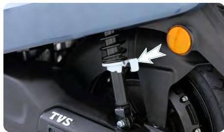
Your Scooter comes with Adjustable Shock Absorber, a first-in-the-industry feature. This allows you to adjust the required level of hardness / softness as per the usage requirement with just a push of a lever. Refer [page No. 74](#) for details
