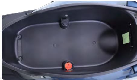
Utility box is located below the seat. Lift the seat by unlocking the seat lock as explained in the previous section, to access the utility box.
