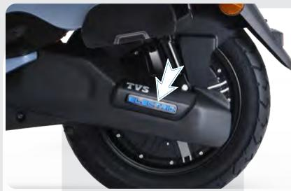
Illuminating logo will display the vehicle type name as 'ELECTRIC' during the vehicle in zero speed conditions. During charging of the vehicle, illuminating logo will blink. The LED color of the illuminating logo is Blue. Illuminating logo is mounted on the swing arm cover as shown above.
