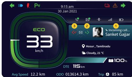
Once mobile app is connected with vehicle instrument cluster, incoming call options (1) will be shown in instrument cluster while you are riding the vehicle as shown above.
