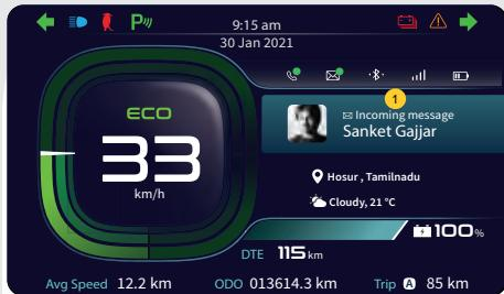
Once mobile phones connected with vehicle instrument cluster, incoming messages notification (1) will be shown in instrument cluster while you are riding the vehicle as shown above.
