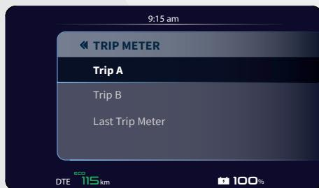
5. You can check the chosen trip meter readings in the display and press center button to reset the trip meter
