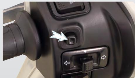
To operate the menu screens on the cluster, the HMI switch is used in the following manner:
