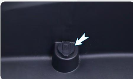
Smart phone charging socket is fitted in your TVS iQube Electric S for charging your smart phone even while you are traveling and it is located in the utility box below the seat assembly. Refer [page No. 25](#) for usage details.
