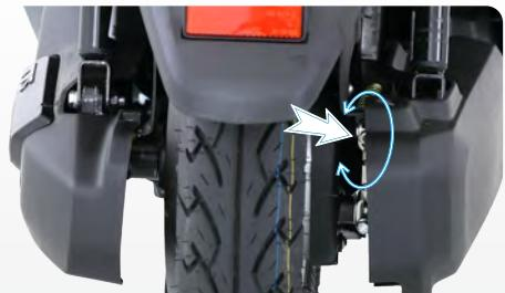
4. Turn the adjuster nut in clockwise direction for reducing free play or in anti-clockwise direction for increasing the free play.
