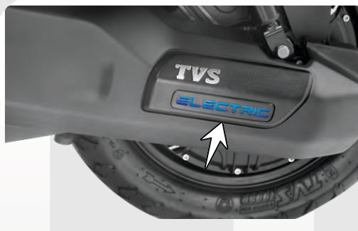
Illuminating logo will display the vehicle type name as 'ELECTRIC' during the vehicle in zero speed conditions. During charging of the vehicle, illuminating logo will blink. The LED color of the illuminating logo is Blue. Illuminating logo is mounted on the swing arm cover as shown above.
