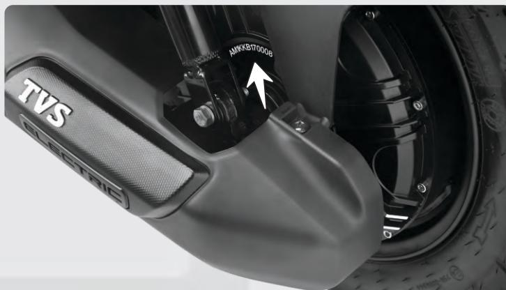
The traction motor serial number is stamped on the hub of the rear wheel assembly. Rotate the rear wheel assembly to read the traction motor number.
