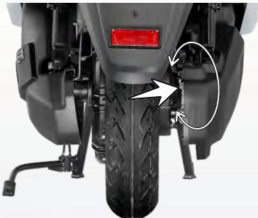
4. Turn the adjuster nut in clockwise direction for reducing free play or in anti-clockwise direction for increasing the free play.
