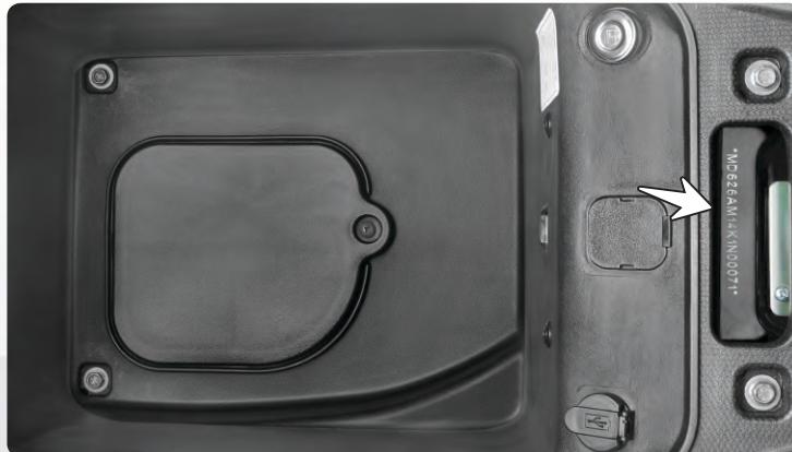
The frame serial number is stamped on the frame, at the rear end below the seat assembly. Open the seat assembly and remove the VIN cover to read the frame number.
