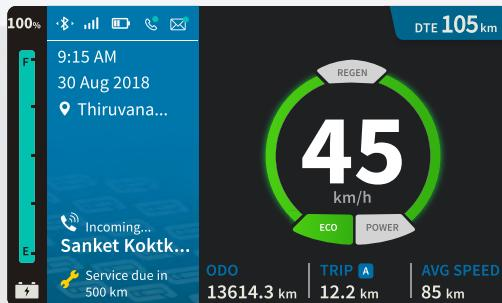
Once Mobile app is connected with vehicle instrument cluster, incoming Call options and messages will be shown in instrument cluster while customer is riding the vehicle as shown above.
