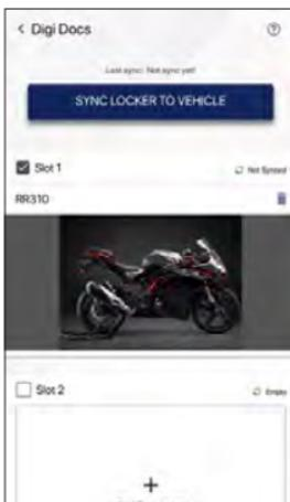
Now the image is ready to transfer to TFT Instrument cluster. Once the TVS Connect app is connected to TFT Instrument cluster the synchronization starts automatically.
