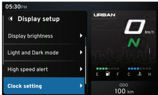
The 'Clock setting' features allows you to adjust the clock timing of your connected instrument TFT cluster. The 'Clock setting' feature has three settings and they are:
