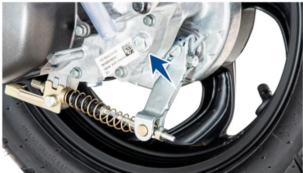
4. Check for the flow of oil from oil level hole. If the level is less (if there is no oil flow), top-up with 'TVS TRU4 SKUUTA oil (SAE 10W30 API-SL, JASO MB)' till the oil just starts to flow out from the oil level hole.
