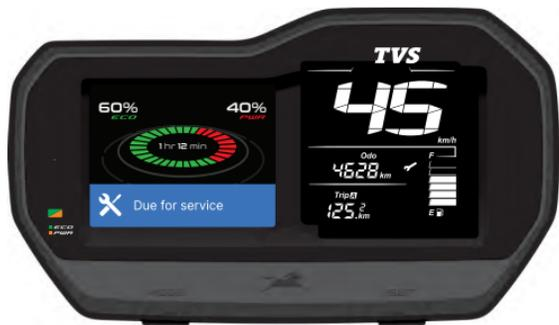
If the service is due, whenever the ignition is turned 'ON', a icon with spanner symbol '🔧' blinks for 10 seconds after the self-check cycle of connected instrument cluster and continue to glow till the vehicle is serviced and the reminder is reset. Get the vehicle serviced at TVS Motor Company Authorised Main Dealer / Authorised Dealer.
