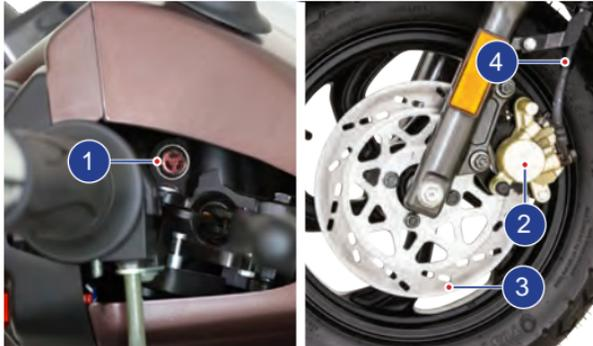
3. Check the master cylinder brake fluid level through the view piece glass (A).
