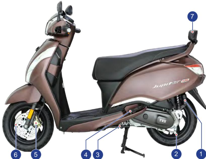
1. Gas filled adjustable rear shockabsorber
