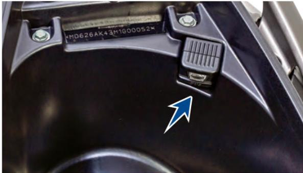
TVS Jupiter 125 comes with utility box light which is located in the utility box of your vehicle (refer page no. 25 for opening seat). The light glows once the seat is opened and gets 'OFF' when the seat closed automatically.
