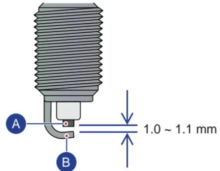
After cleaning and checking the gap, reinstall the spark plug and tighten by hand to avoid cross threading. Finally tighten using spark plug spanner. Do not over tight or cross thread the spark plug. After reassembling the plug fix back the suppressor cap and ensure its proper fitment.
