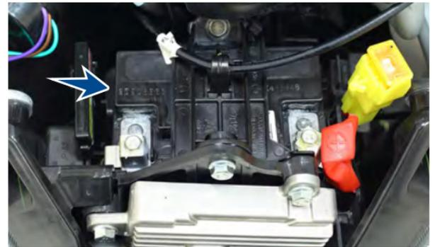
2. While connecting the terminals, observe the correct polarity. Connect the red wire to the '+' terminal and black wire to the '-' terminal of the battery.
