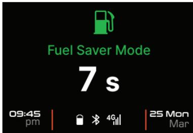
The IntelliGO indicator starts glowing during the engine stop to indicate you that the vehicle has stopped due to 'IntelliGO' system.
